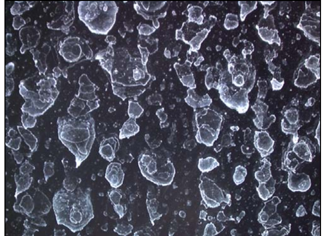
Figure 10: Close up view of typical concrete runoff deposits on glass. These deposits begin to react with glass upon evaporation of the runoff droplets resting on the glass
