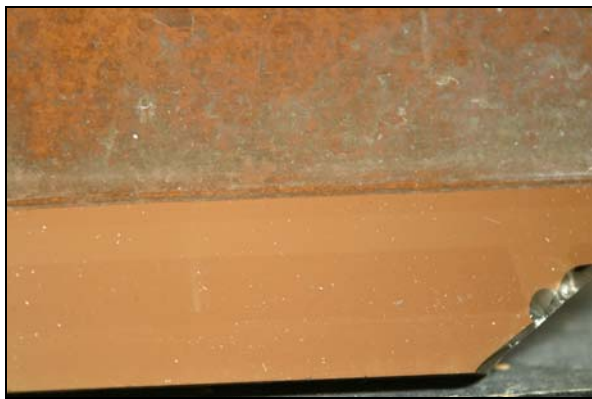
Figure 12. Concrete runoff deposits on coated glass unit removed from an existing glazing installation. Note the line of demarcation at point where glass was protected by framing.
