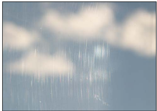
Figure 8: Another example of a window glass surface where the observed scratches are indicative of cleaning in the absence of an experienced professional.
